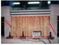
Fig. 2 Column shear failure in as observed in [3]
